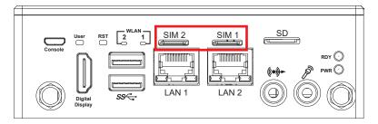
There are two external Nano SIM cards M1 and SIM2 are assigned for mini PCIe slot and M.2 key B slot respectively offers wireless communication capability to the system.
