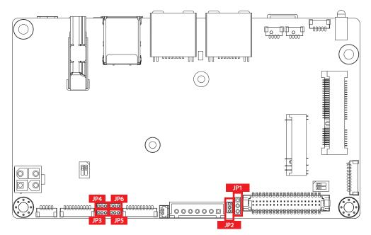
To "close" a jumper, you connect the pins with the clip. To "open" a jumper, you remove the clip. Sometimes a jumper will have three pins, labeled 1, 2 and 3. In this case you would connect either pins 1 and 2, or 2 and 3.
