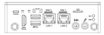
In Vecow EIC-2000 series, all I/O connectors are located on the front and top panels. Most of the general connections to computer devices, such as USB, COM, LAN, Console port, Reset button, audio/mic, digital display indicators are placed on the front panel.
