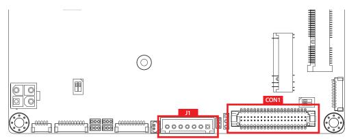
EIC-2000 supports dual-channel 24-bit LVDS display, up to 1920 x 1080 pixels resolution. The pin assignments of CON1 are listed in following table. The panel power level can be changed by JP1, 5V or 3.3V.
