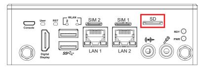
The external Micro SD card provides additional storage expansion. It is located behind the cover-plate on the bottom panel. If you would like to replace or insert the card, it MUST be ensure the system is powered off.
