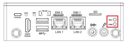
There are two LEDs defined system power up (green LED) and system work (yellow LED) respectively. When the system power is ready, the top LED (green LED) will be lighted up stably, it means the power of system is already powered up. When the system boot up, the bottom LED (yellow LED) will be flashed, it means the system boot up successfully.
