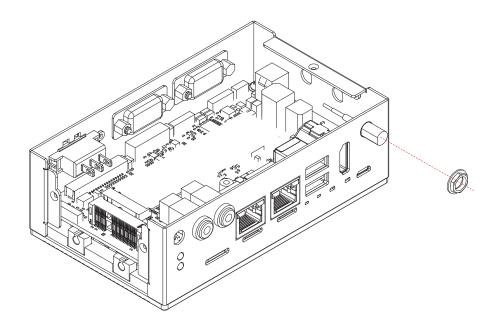
**Step 3** Fasten washer on the antenna cable connector.
