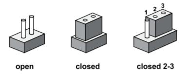
The Pin Header JP1 Jumper select can be changed panel power level for panel, and JP2 Jumper select can be changed power level of backlight PWM and enable. As following configuration table. The two jumpers default setting are shorted Pin 1 and Pin 2.
