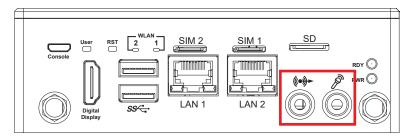
There two 3.5 mm audio jacks for line-out and mic in function on the front side of EIC-2000. The function is line-out and mic in from left jack to right jack.
