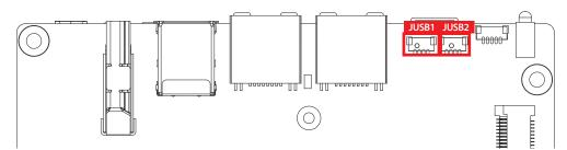
EIC-2000 is equipped with an USB2.0 header for reserve function.
