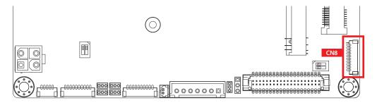
There is a 6-bit GPIO and one I2C in connector on the Top side. Each GPIO channel can be confguration GPI or GPO. The all signal with voltage 3.3v level.
