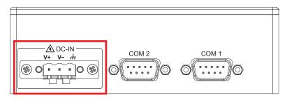
There two COM ports (COM1 and COM2), it can be configured for RS-232, RS-422, or RS-485 by GPIO control with auto flow control communication. The default definition of COM1 and COM2 is RS-232; if you want to change to RS-422 or RS-485, you can find the setting in software.
