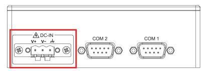
EIC-2000 supports 9V to 55V DC wide range power input by terminal block on the top side.
