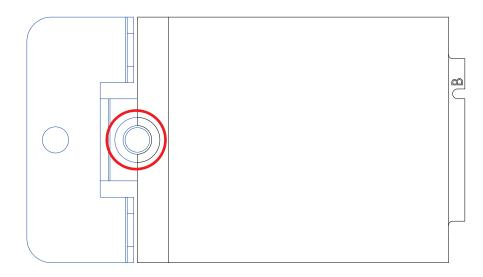
**Step 2** Install M.2 card into the M.2 slot and fasten PHILLIPS-M3x4L screw.
