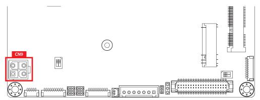
EIC-2000 supports 9V to 55V DC power input by wire to board cable to terminal block connector on the top side.
