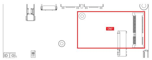
There is a Mini PCIe slot supported with USB 2.0 and PCIE Gen3 signal in EIC-2000. The PCIe signal only option one slot, either Mini PCIe slot or M.2 key B slot. If the Mini PCIe slot can work normally by PCIe signal, the SW2.2 must be switched to "off".
