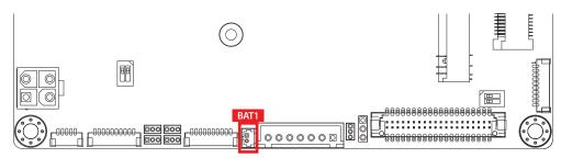
The real-time clock of EIC-2000 is powered by a lithium battery. It is equipped with muRata CR2032 210mAh lithium battery. It is recommended that you not replace the lithium battery on your own. If the battery needs to be changed, please contact Vecow RMA service team.
