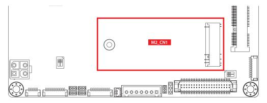
There is a M.2 key B supported with USB 3.0 and PCIE Gen3 signal in EIC-2000. The PCIe signal only option one slot, either Mini PCIe slot or M.2 key B slot. If the M.2 Key B slot can work normally by PCIe signal, the SW2.2 must be switched to "on".
