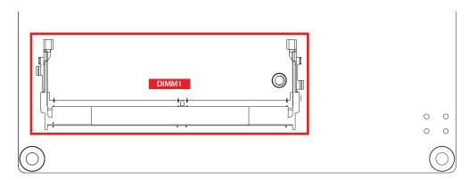
The DIMM1 only for EDM-G-IMX8M-PLUS module.
