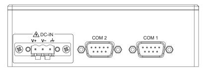
On the Rear panel side, there are three connectors terminal block of power input and 2 DB-9 Ports in EIC-2000 Series.
