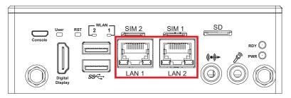
There are two Ethernet ports auto-sensing 10/100/1000 Mbps in RJ45 connectors on the front side of EIC-2000 series. Both are powered by RTL8211FI-CG Ethernet PHY. The Pin out of LAN1 and LAN2 are listed as following chart.
