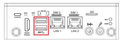
The USB interface supports 5 Gbps transfer rate complied with Super speed USB specification Rev. 3.0. The top port is a pure USB port, the bottom port can be changed OTG function and pure USB by DIP Switch SW2.
